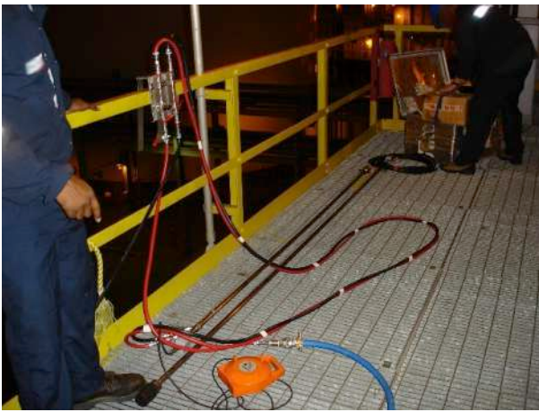
Assembly of Gold Cup system showing cooling water hoses and regulator panel
